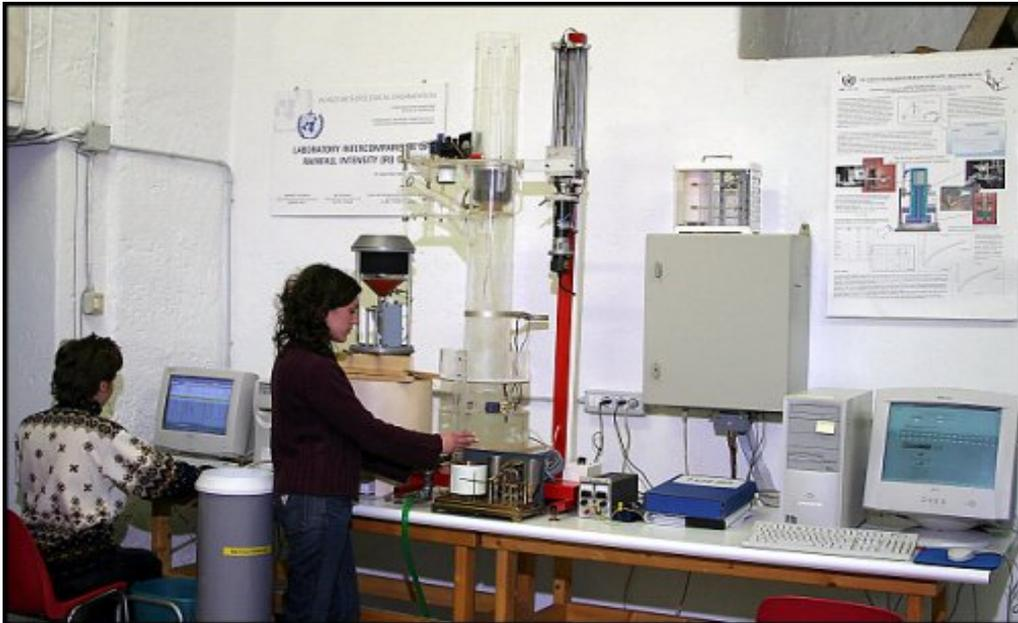
**Fig. 12:** The Qualification Module for Rainfall Intensity Measurement Instruments developed at the University of Genova, and used in the laboratory calibration phase.
