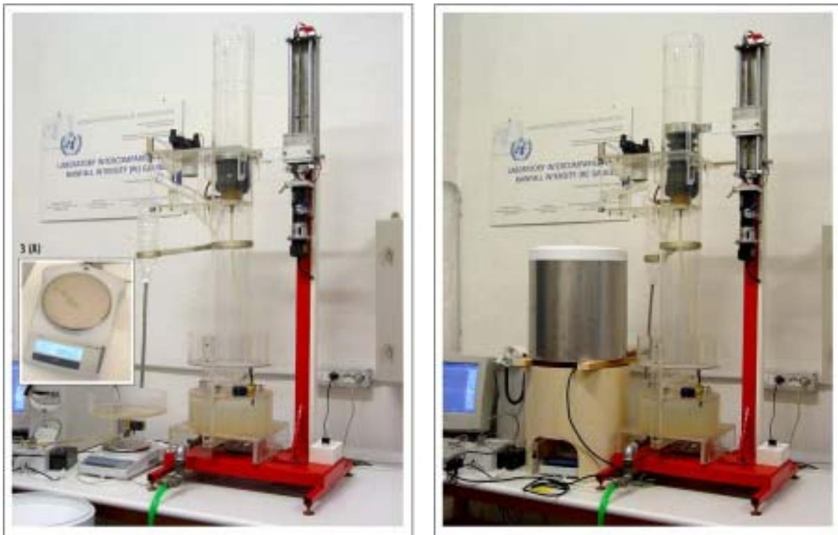
**Figure 3:** Present configuration of the QM-RIM with (right) and without (left) a RI gauge under test. The inner rectangle also shows a close view of the precision balance, while on the right hand side the plastic support for gauges can be seen.
