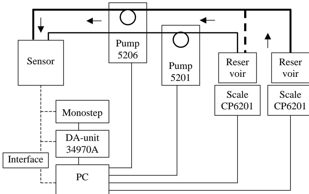
**Figure 5:** Sketch of the KNMI calibration setup used for the WMO laboratory intercomparison of rainfall intensity gauges and a photograph of the setup with the KNMI precipitation gauge.
