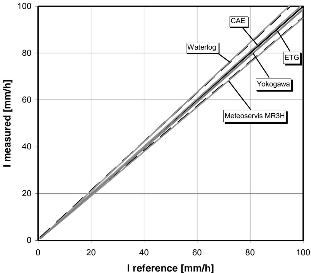
**Figure 9b:** Ensemble of calibration curves for corrected TBRG (dashed lines indicate  $\pm 5\%$ ) over the range of reference rainfall intensities from 0 to  $100 \text{ mm}\cdot\text{h}^{-1}$ .
