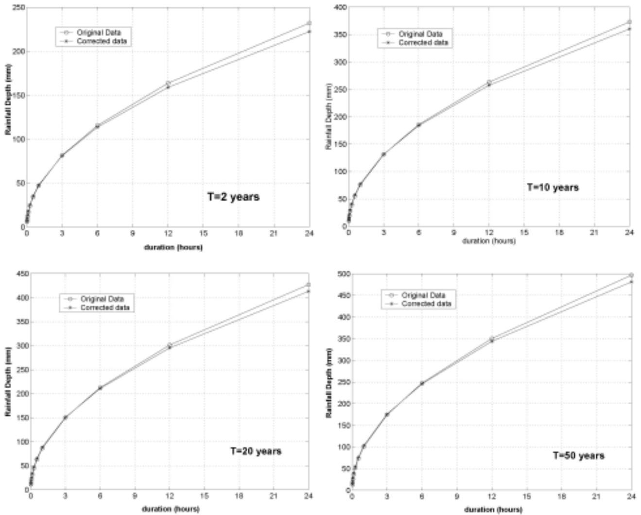
Figure 1: Original and corrected DDF curves for a sample station at various return periods.
