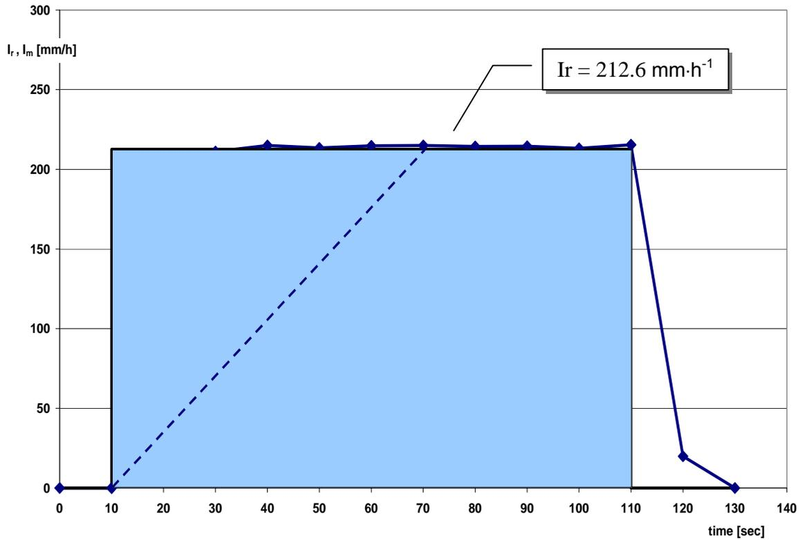
**Figure 12:** Step response for the Meteoservis MRW500 weighing gauge, showing a delay in sensing the rain rate signal of about 20 seconds. The dotted line shows the response curve to be reported by an ideal RI-gauge, based on the defined averaging interval of 60 s.
