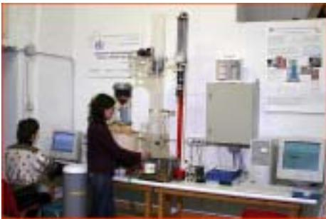
**Head losses on hydraulic devices.** The Laboratory is equipped with a hydraulic system for flow measurements and the assessment of local head losses caused by devices (valves, filters, etc.) conveniently supervised.
