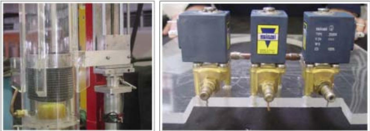
**Figure 4:** Close view of the cylindrical bellows which allows varying the water level in order to produce different water heads. The top of the bellows is connected to a motor with encoder controlled software. On the right hand side there are three electrovalves that allow to combine different nozzles diameters in order to produce a wide range of water flow rates.
