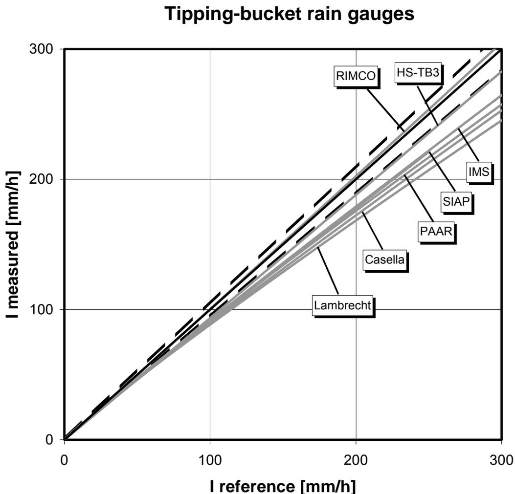
**Figure 8:** Ensemble of response curves for the non-corrected TBRG (dashed lines indicate  $\pm 5\%$ ).
