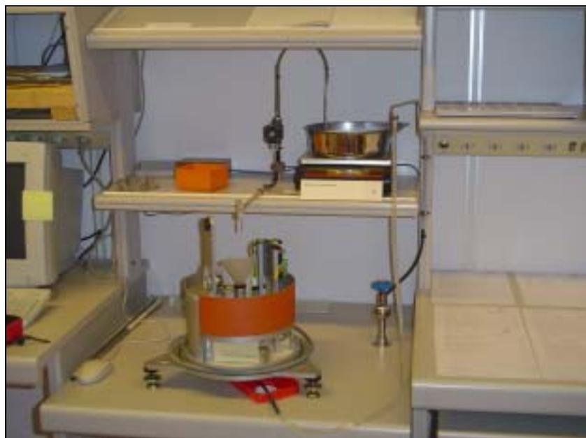
**Figure 3:** The calibration setup for the KNMI precipitation gauge at the laboratory of KNMI.
