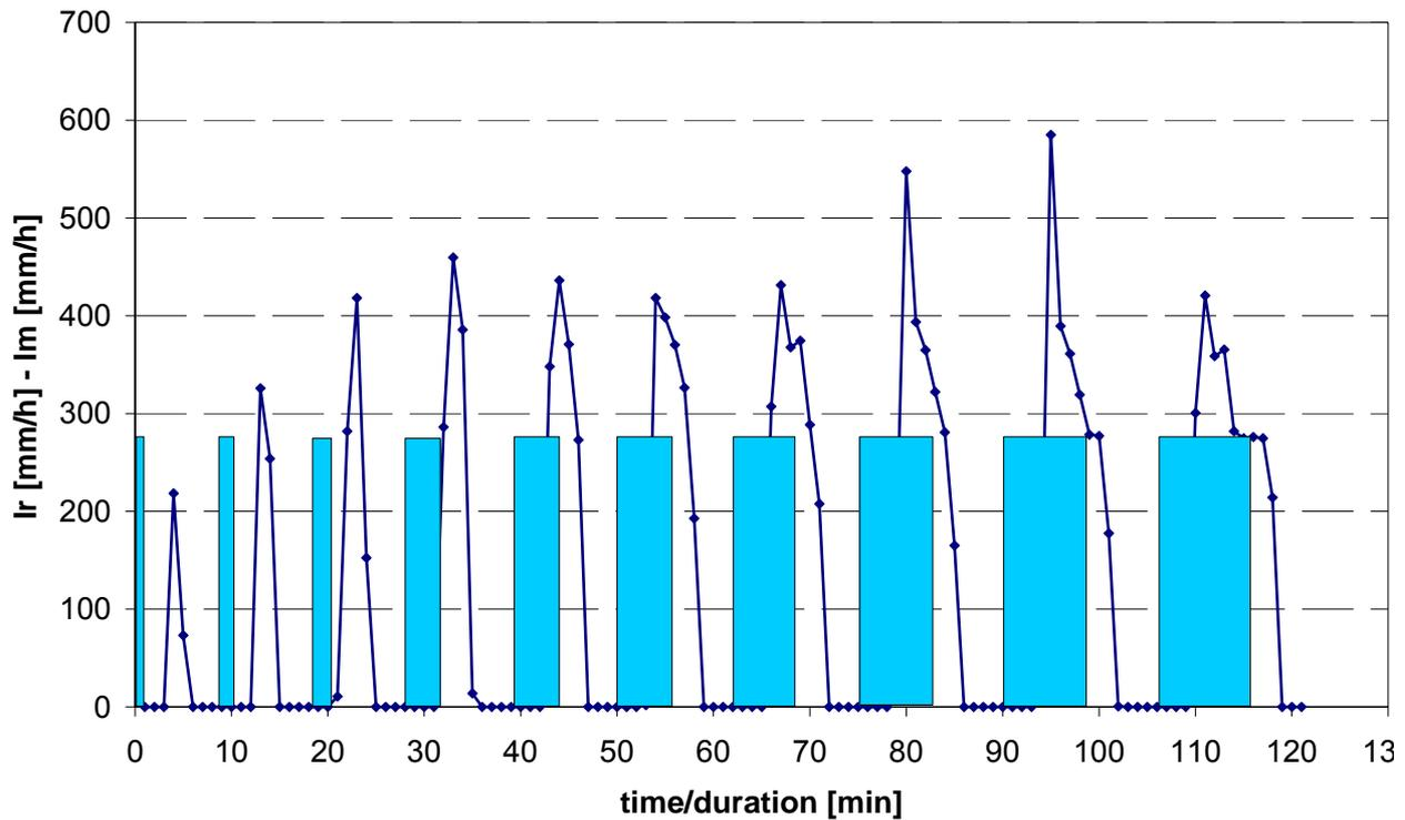
**Figure 15:** Step response for the OTT Pluvio weighing rain gauge, at varying pulse duration but the same reference intensity. The data points indicate the rain intensity values reported by the instrument with a resolution of one minute.
