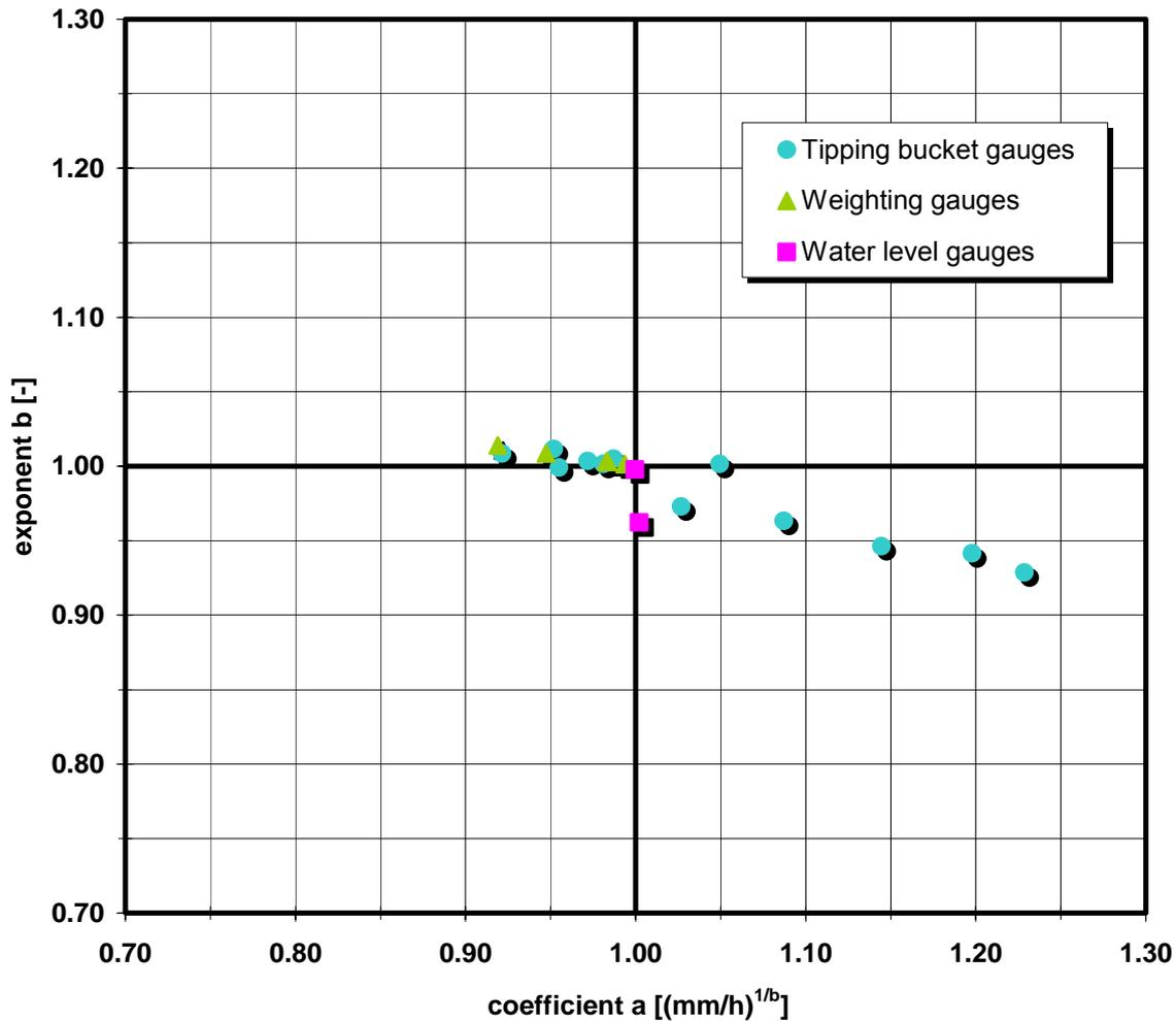
**Figure 18:** Scatter plot of the parameters' values for the power law calibration curve of all the instruments analyzed. The perfect rain intensity gauge is associated with the pair (a, b) = (1, 1).
