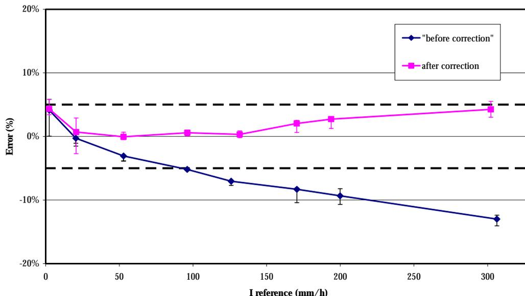
**Figure 10:** Sample comparison between the original and corrected curve for the CAE instrument.
