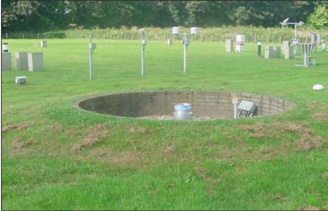
**Figure 2:** A picture of the operational precipitation gauge setup used by KNMI.
