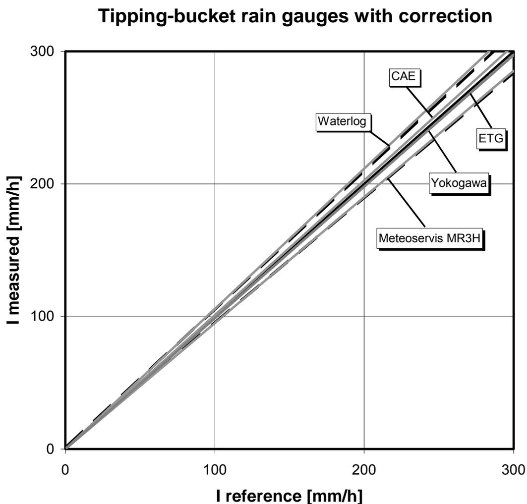
**Figure 9a:** Ensemble of calibration curves for corrected TBRG (dashed lines indicate  $\pm 5\%$ ) over the range of reference rainfall intensities from 0 to 300  $\text{mm}\cdot\text{h}^{-1}$ .
