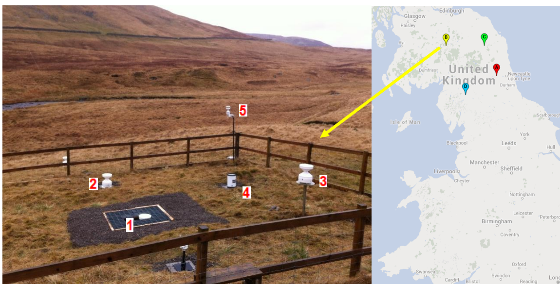
Figure 1: Talla Reservoir research station, Scottish Borders. Elevation: 430m. Identical aerodynamic rain gauges (ARG100s) are mounted at different heights: reference pit gauge (1), ground-mounted gauge (2), 1-metre mounted gauge (3). There is also a ground mounted straight-sided gauge (4) and wind speed measurement at two metres (5) This upland site is situated at the top of a valley running east-west, with strong winds observed. (Picture by M.Pollock, April 2015. Site provided by University of Dundee).
