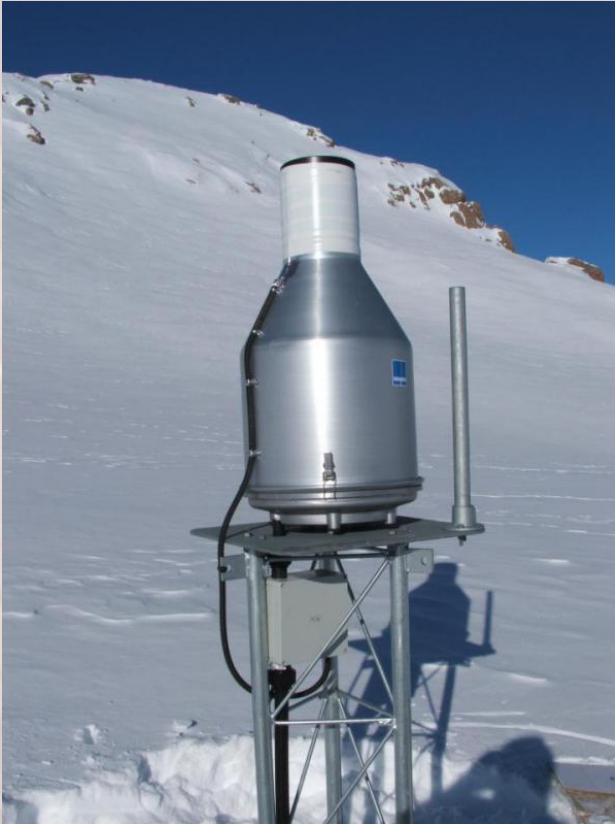
Geonor 600 mm – vibrating wires gauge
