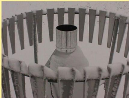
This study focuses on the single Alter shielded Geonor T200B weighing gauge.
