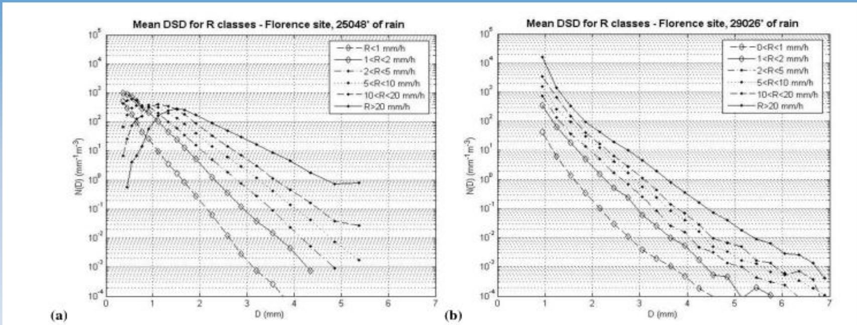
Co-located DSD measurements made by an impact Joss-Waldvogel disdrometer (a) and a X-band radar disdrometer (b) in Florence (Caracciolo et al., 2008)
