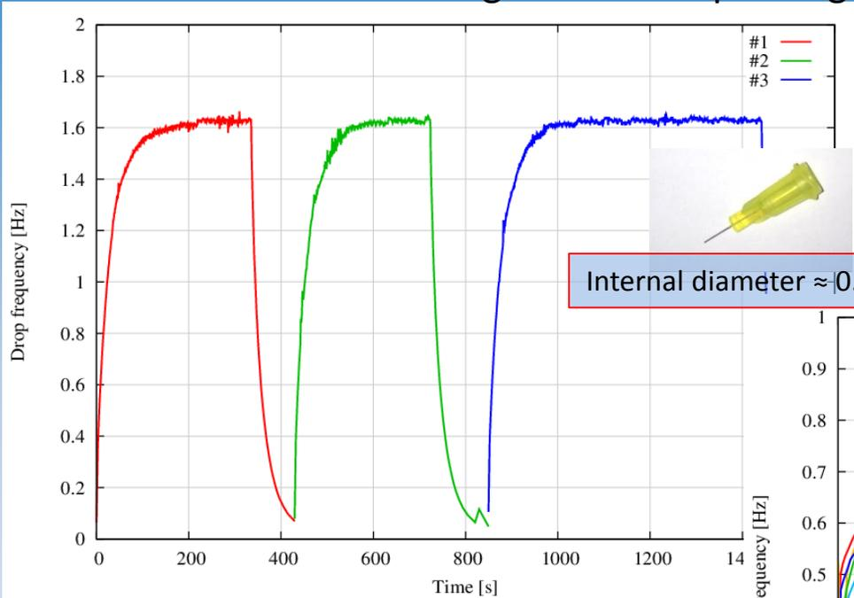
Since the nozzle dispensing is realized by imposing constant flow rate values, *a constant drops time period (or frequency) corresponds to equally sized drops generation.*
